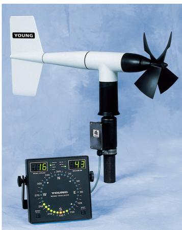
A variety of inputs and outputs including 4-20 mA, Serial (RS-485), and Voltage are standard on the Wind Tracker. Alarms for both wind speed and wind direction are standard.
