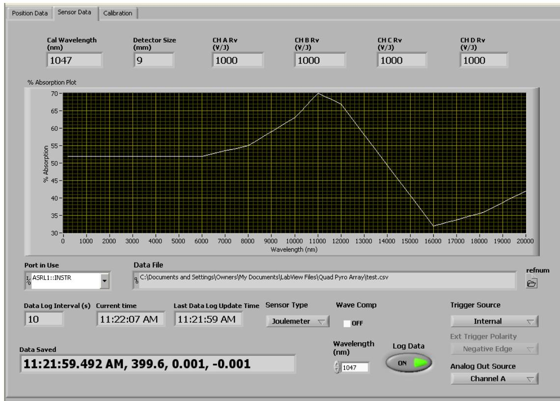
The Sensor Data Display has Controls and Indicators related to the sensor. The sensor information is read from the sensor memory on program startup.
