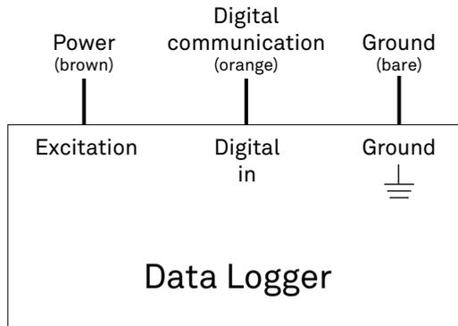
Figure 3 Wiring diagram
