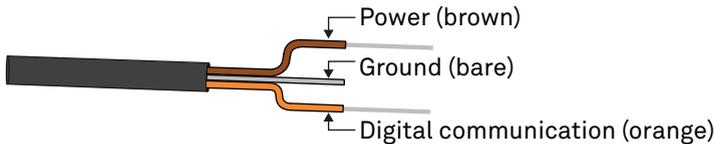
Figure 2 Pigtail wiring
