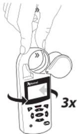
Place the base of the Kestrel on a flat surface at least 3 feet from any large metal objects.
