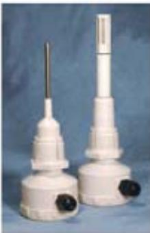
The sensor assembly is securely mounted in a convenient junction box that fits YOUNG radiation shields. For special applications, the temperature probe is available with various output options. The 4-20 mA current output is useful in high noise, industrial settings or for long cable lengths. The 0-1 VDC option provides a calibrated voltage output signal. Low power circuitry makes it ideal for field studies and remote data-logging applications.
