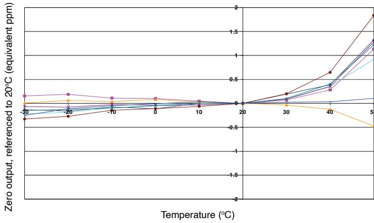
Figure 1 shows the variation in zero output caused by changes in temperature, expressed as ppm gas equivalent, referenced to zero at 20°C.
