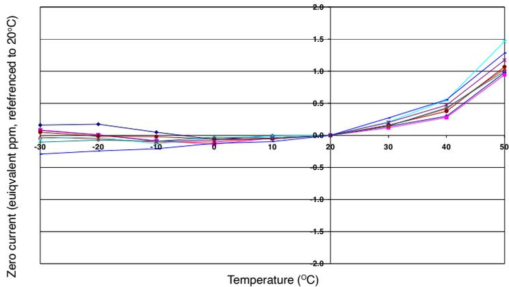
Figure 2 shows the variation in zero output caused by changes in temperature, expressed as ppm gas equivalent, referenced to zero at 20°C.
