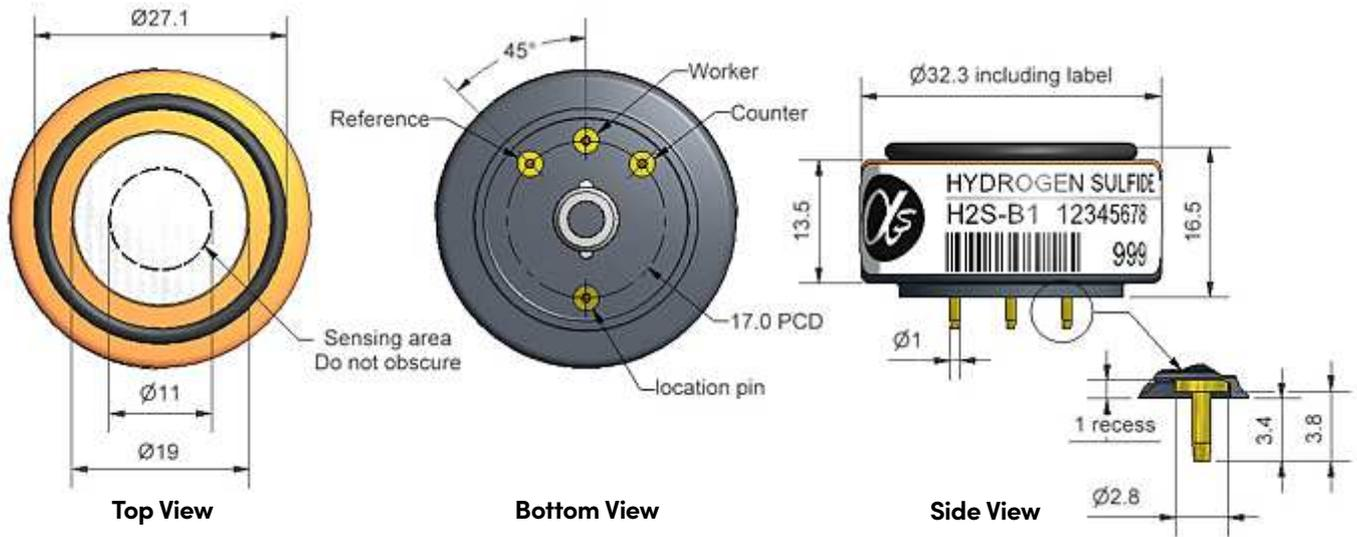
Dimensions are in millimetres ( $\pm 0.1$  mm).
