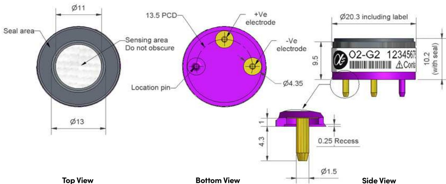
Dimensions are in millimetres ( $\pm 0.15$  mm).
