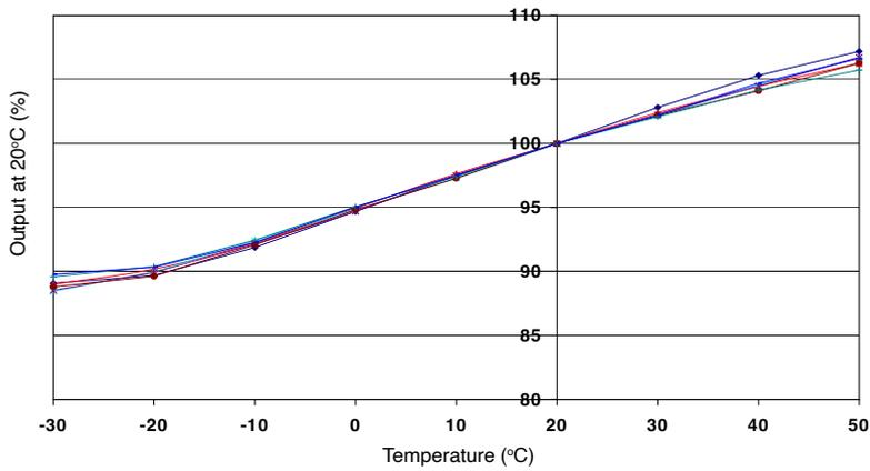
This graph shows the variation in sensitivity caused by changes in temperature.
