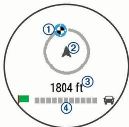
The destination indicator ① shows the direction of your destination relative to the direction you are moving ②. When the destination indicator appears at the top of the circle, you are heading toward your destination. The remaining distance to your destination ③ appears below the circle. The progress bar ④ shows your progress toward your destination.
