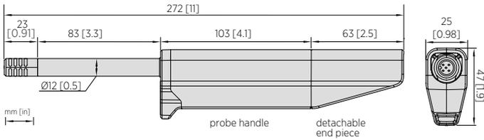
Figure 1 HMP80N dimensions, side and bottom view
