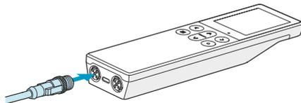
3. Connect the probe to the M12-5F end of the probe connection cable.
