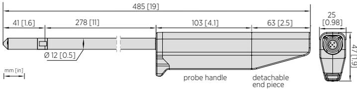
Figure 2 HMP80L dimensions, side and bottom view
