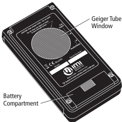
tube. The small radiation symbols on the front label (5) and the end label (9) indicate the center of the Geiger tube.
