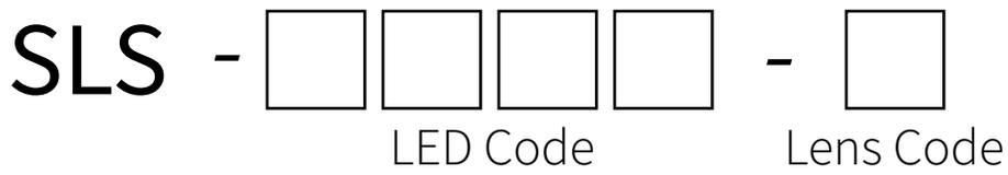
For example, SLS-0104-B is a light source with a 1W green emitter and 15-degree collecting optics.
