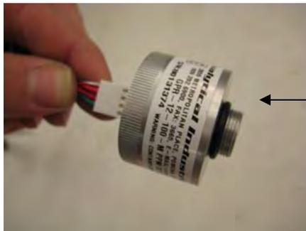
Hold the sensor pressed against the contact pins inside the housing
