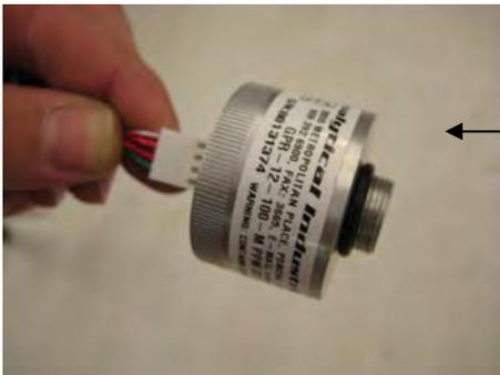
Hold the sensor in your hand in air and perform air calibration
