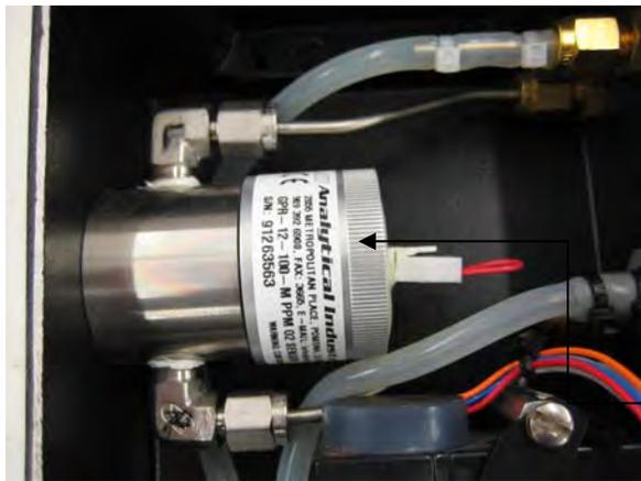
Unscrew the old sensor and screw in the new sensor finger tight
