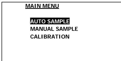
This screen shows various options available. You can use the UP and DOWN arrow keys to move the cursor and highlight the desired function. After moving the cursor to the desired function, you can press ENTER to go to that function.
