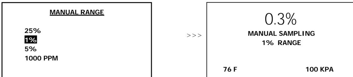
If the oxygen value goes above the 1%, display will not shift to the next higher range. Instead, when the oxygen reading exceeds 110% of the upper limit of the current range, an OVER RANGE warning will be displayed.
