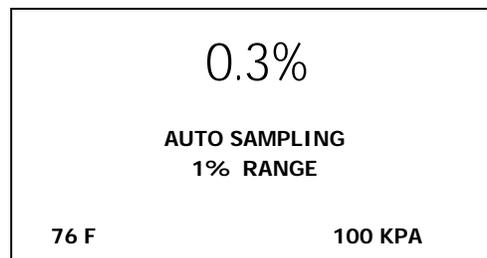
The display will shift to the next higher range when the oxygen reading exceeds 99.9% of the upper limit of the current range. The display will shift to the next lower range when the oxygen reading drops to 85% of the upper limit of the next lower range.
