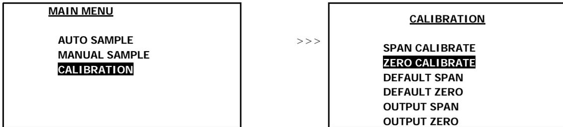
4. Advance the reverse shade cursor using the ARROW keys to highlight ZERO CALIBRATE.
