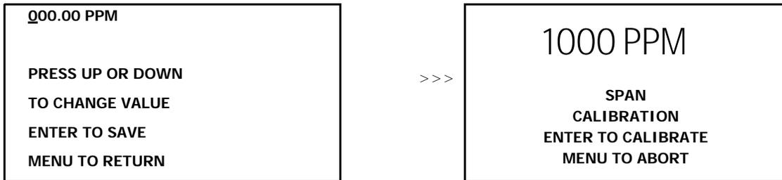
13. By using the UP or DOWN arrow keys, enter the appropriate digit where the cursor is blinking
