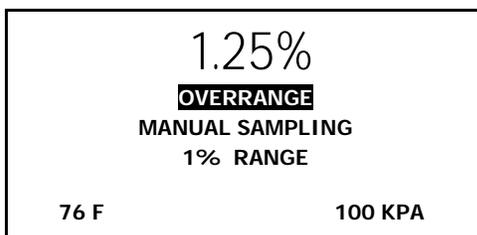
Once the OVER RANGE warning appears the user must advance the transmitter to the next higher range.
