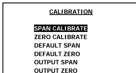
8. After selecting the SPAN CALIBRATION, enter appropriate span gas value.
