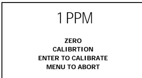
6. Wait until the analyzer reading stabilizes (depending on the history of the sensor, it may take a few minutes to several hours) and then press the ENTER key to calibrate (or MENU key to abort).
