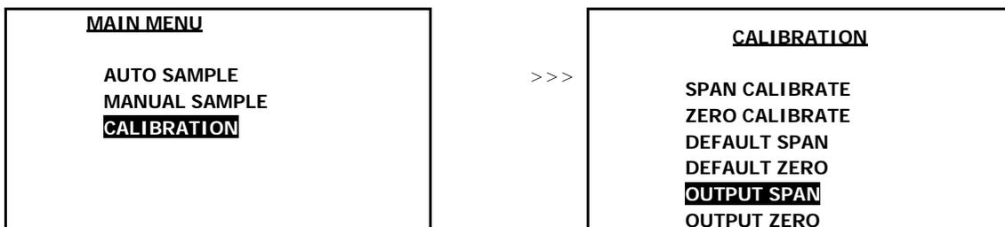
4. Advance the reverse shade cursor using the ARROW keys to highlight DEFAULT SPAN.
