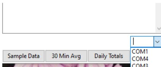
When you have connected to the correct COM#, the software will say “Connected”.
