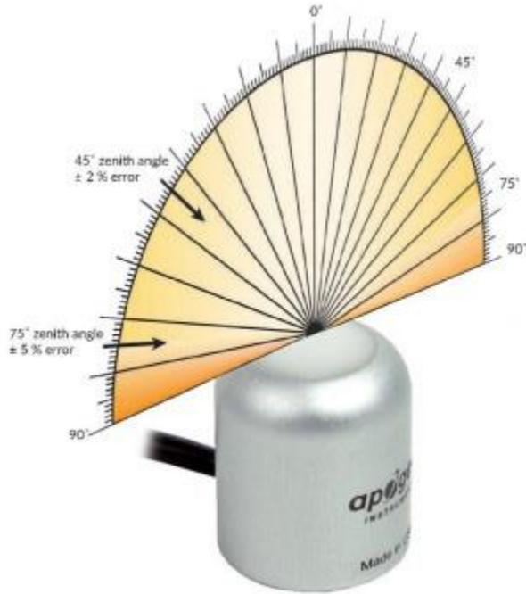
Directional, or cosine, response is defined as the measurement error at a specific angle of radiation incidence. Error for Apogee MQ-600 series ePAR Sensor is approximately ± 2 % and ± 5 % at solar zenith angles of 45° and 75°, respectively.
