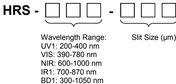
For example, HRS-VIS-010 is a spectrometer with a wavelength range of 390-780nm and a 10 µm slit size.
