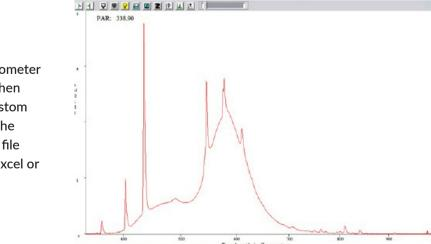
The detector collects light for the spectroradiometer via fiber-optic cable. The spectroradiometer then transmits its measurements to a PC where custom software (included) displays the spectrum of the light source. Live data can be saved as a data file suitable for work in other programs, such as Excel or SigmaPlot.
