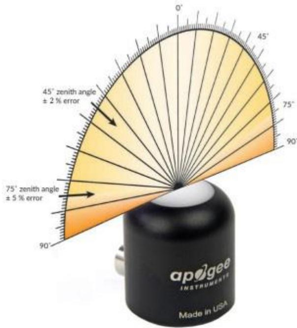
Directional, or cosine, response is defined as the measurement error at a specific angle of radiation incidence. Error for Apogee S2 series PAR-FAR sensors is approximately ± 2 % and ± 5 % at solar zenith angles of 45° and 75°, respectively.
