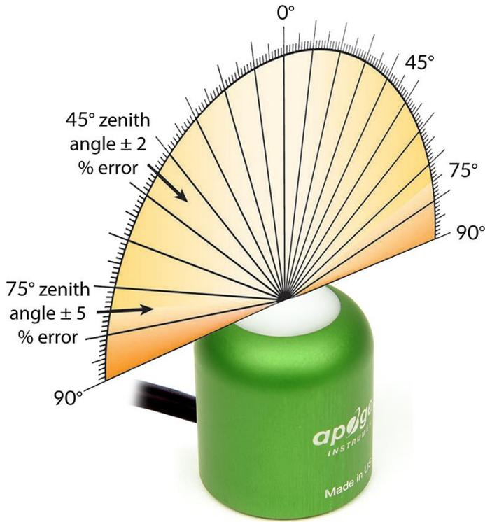
Directional, or cosine, response is defined as the measurement error at a specific angle of radiation incidence. Error for Apogee SE series photometric sensors is approximately ± 2 % and ± 5 % at solar zenith angles of 45° and 75°, respectively.
