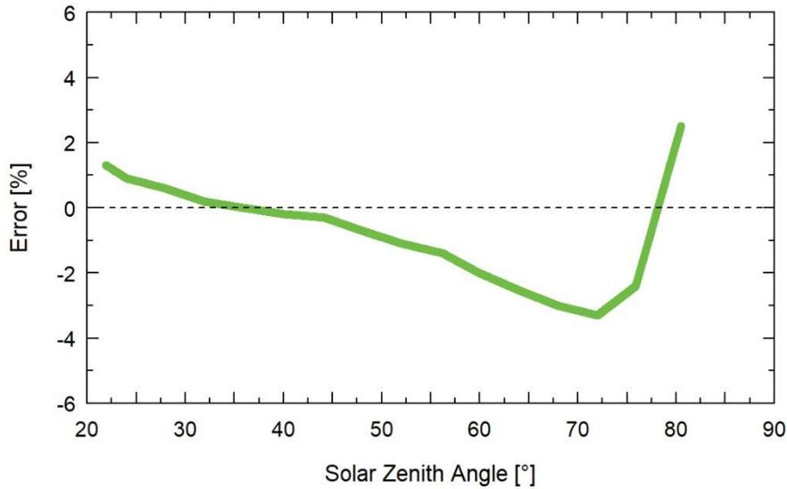
Cosine response measurements were made by direct side-by-side comparison to the mean of four reference SE-100 photometric sensors.
