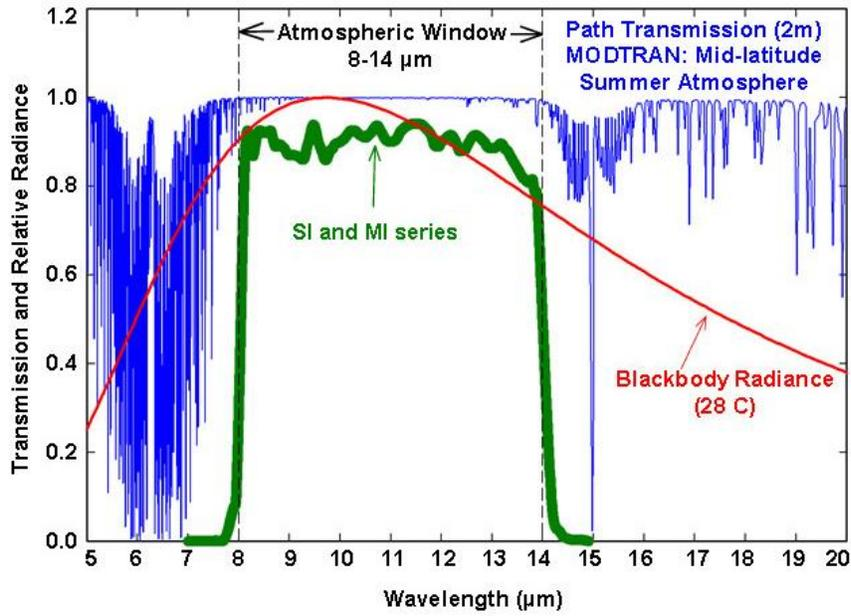
Spectral response of SIL series infrared radiometers. Spectral response (green line) is determined by the germanium filter and corresponds closely to the atmospheric window of 8-14 µm, minimizing interference from atmospheric absorption/emission bands (blue line) below 8 µm and above 14 µm. Typical terrestrial surfaces have temperatures that yield maximum radiation emission within the atmospheric window, as shown by the blackbody curve for a radiator at 28 C (red line).
