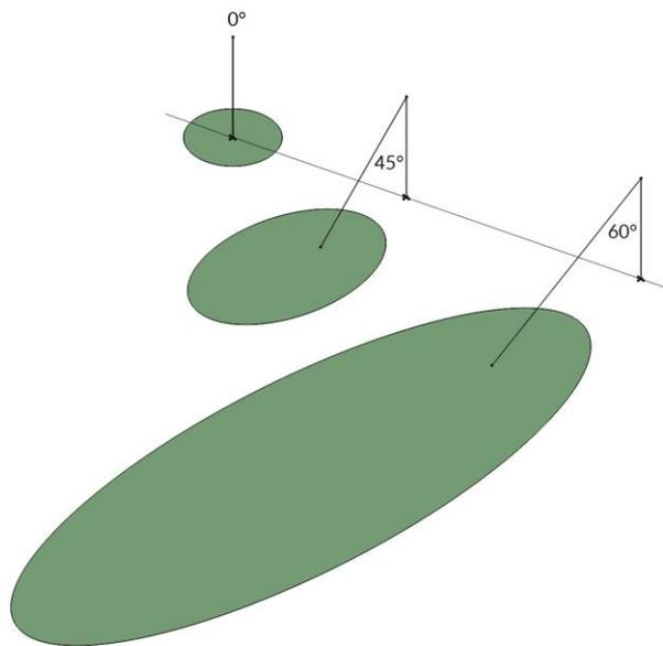
A simple FOV calculator for determining target dimensions based on infrared radiometer model, mounting height, and mounting angle, is available on the Apogee website: <https://www.apogeeinstruments.com/irr-calculators>.
