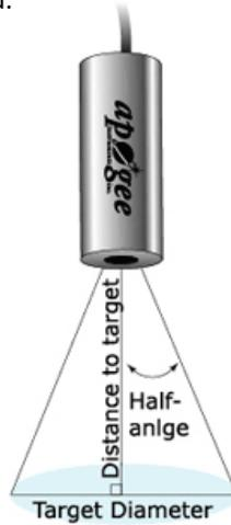
Sensor FOV, distance to target, and sensor mounting angle in relation to the target will determine target area. Different mounting geometries (distance and angle combinations) produce different target shapes and areas, as shown below.
