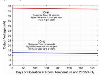
Long-term stability (output voltage decrease over time) of Apogee SO-400 series oxygen sensors. The response time and signal decrease for both series are also listed.
