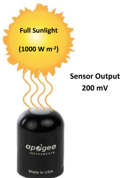
Example of total shortwave radiation measurement with an Apogee SP-110 pyranometer. Full sunlight yields total shortwave radiation on a horizontal plane at the Earth's surface of approximately  $1000 \text{ W m}^{-2}$ . This yields an output signal of 200 mV. The signal is converted to shortwave radiation by multiplying by the calibration factor of  $5.0 \text{ W m}^{-2} \text{ per mV}$ .
