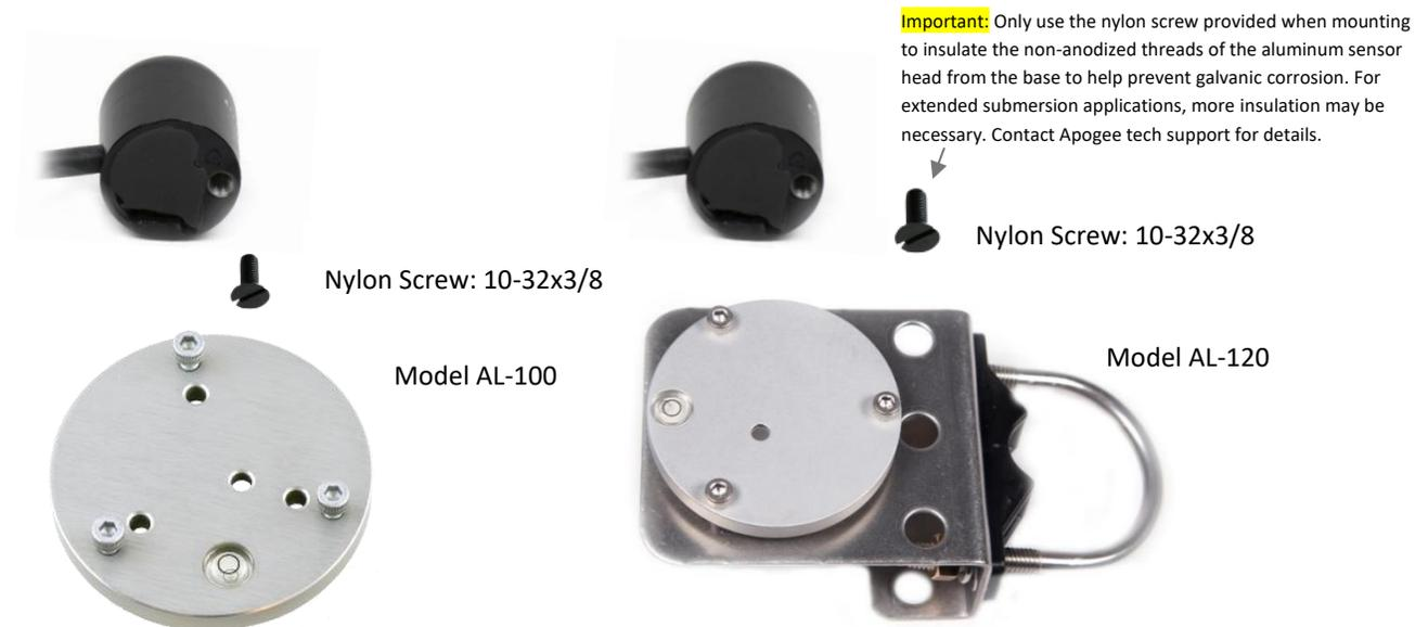
To minimize azimuth error, the sensor should be mounted with the cable pointing toward true north in the northern hemisphere or true south in the southern hemisphere. Azimuth error is typically less than 1 %, but it is easy to minimize by proper cable orientation.
