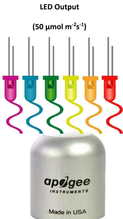
Example of photon flux density measurement with an Apogee model SQ-640 Quantum Light Pollution Sensor. The LED in this example Full yields a photon flux density on a horizontal plane of  $50 \mu\text{mol m}^{-2} \text{ s}^{-1}$ . This yields an output signal of 50 mV. This signal is converted to photon flux density by multiplying by the calibration factor of  $1 \mu\text{mol m}^{-2} \text{ s}^{-1} / \text{mV}$ .
