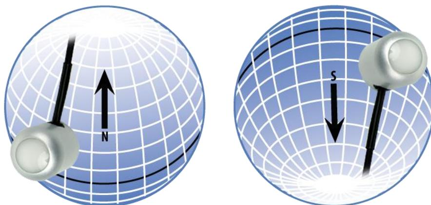
In addition to orienting the cable to point toward the nearest pole, the sensor should also be mounted such that obstructions (e.g., weather station tripod/tower or other instrumentation) do not shade the sensor. **Once mounted, the blue cap should be removed from the sensor.** The blue cap can be used as a protective covering for the sensor when it is not in use.
