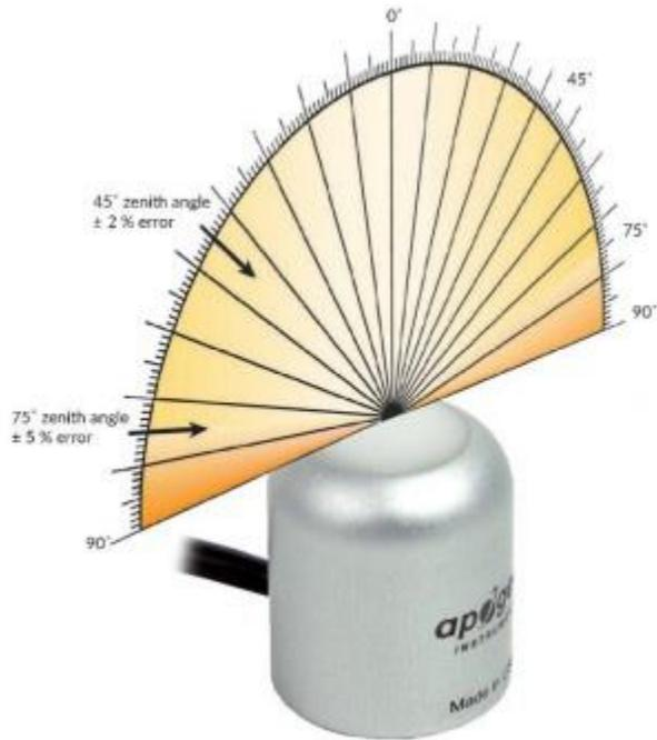
Directional, or cosine, response is defined as the measurement error at a specific angle of radiation incidence. Error for Apogee SQ-600 series Quantum Light Pollution Sensor is approximately ± 2 % and ± 5 % at solar zenith angles of 45° and 75°, respectively.
