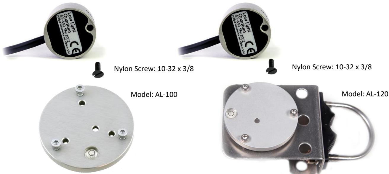
To minimize azimuth error, the sensor should be mounted with the cable pointing toward true north in the northern hemisphere or true south in the southern hemisphere. Azimuth error is typically less than 0.5 %, but it is easy to minimize by proper cable orientation.
