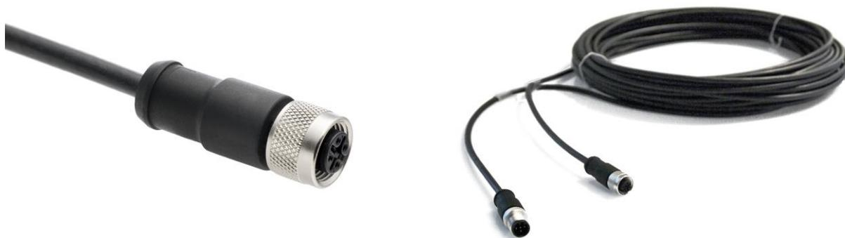
**Figure 8.1.1** *On the left the SR05-A1 cable with M12-A female connector on sensor end. The cable is non-stripped on the other end. Its length is 3 metres standard and available in 10 and 20 metres too. On the right Hukseflux extension cable with connector pairs, with male and female M12-A connectors, available in 10 and 20 metres.*
