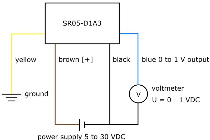
**Figure 5.7.1** Electrical diagram of the connection of SR05-D1A3 to a typical voltmeter or datalogger with the capacity to measure voltage signals. SR05-D1A3 operates on a supply voltage of 5 to 30 VDC.
