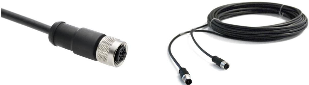
**Figure 9.1.1** *On the left the SR05 cable with M12-A female connector on sensor end. The cable is non-stripped on the other end. Its length is 3 metres standard and available in 10 and 20 metres too. On the right Hukseflux extension cable with connector pairs, with male and female M12-A connectors, available in 10 and 20 metres.*
