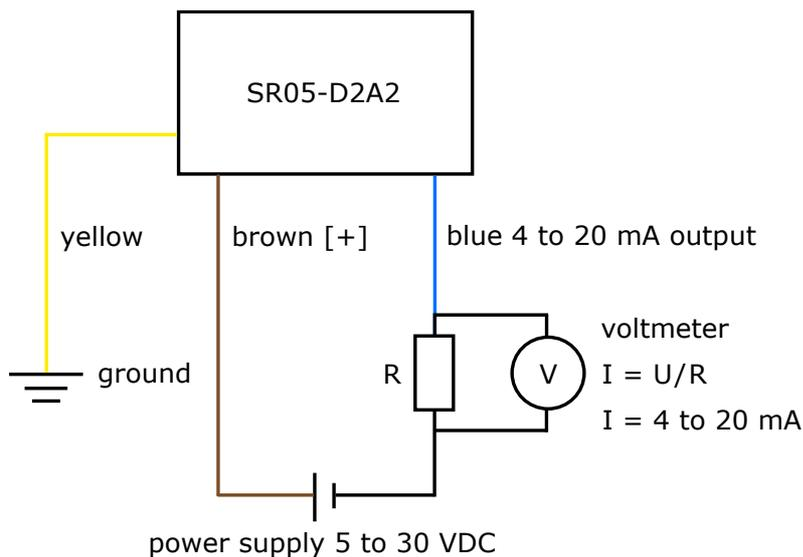
**Figure 5.8.2** Electrical diagram of the connection of SR05-D2A2 to a typical voltmeter or datalogger with the capacity to measure voltage signals. Usually a 100 Ω shunt resistor (R) is used to convert the current to a voltage. SR05-D2A2 operates on a supply voltage of 5 to 30 VDC.
