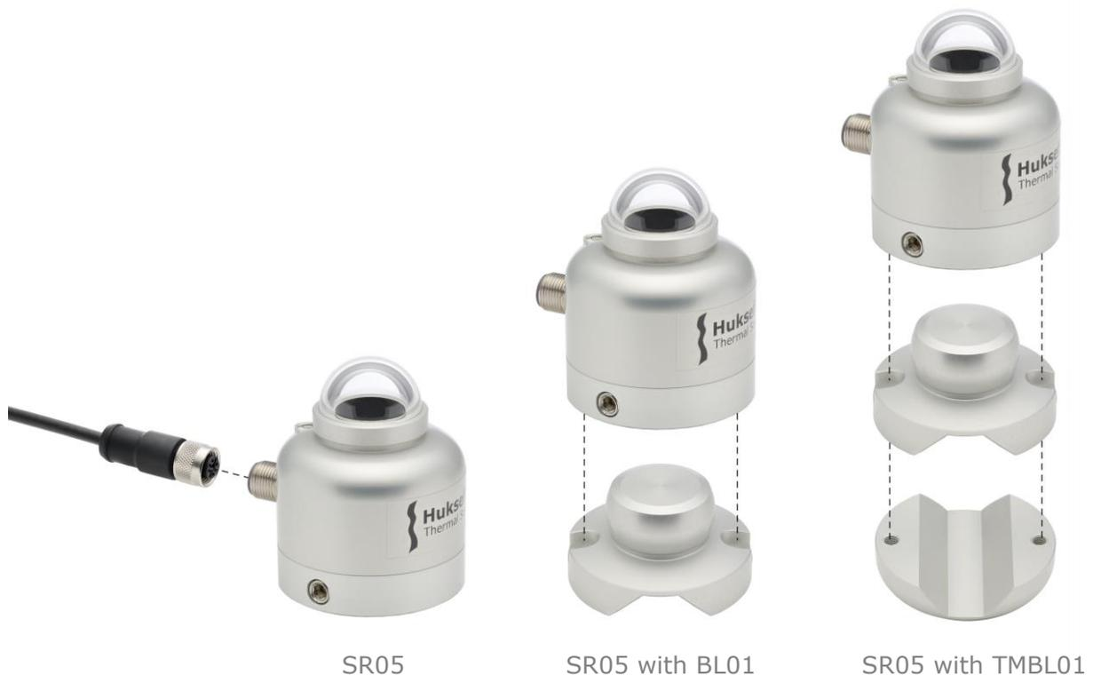
**Figure 5.2.1** From left to right: SR05 in its standard configuration with 3 metre cable; with optional ball levelling for easy mounting and levelling on a (non-)horizontal surface; with optional ball levelling and tube mount for easy installation on a 25 to 40 mm diameter tube. Mounting bolts are included with the ball levelling and / or tube mount.
