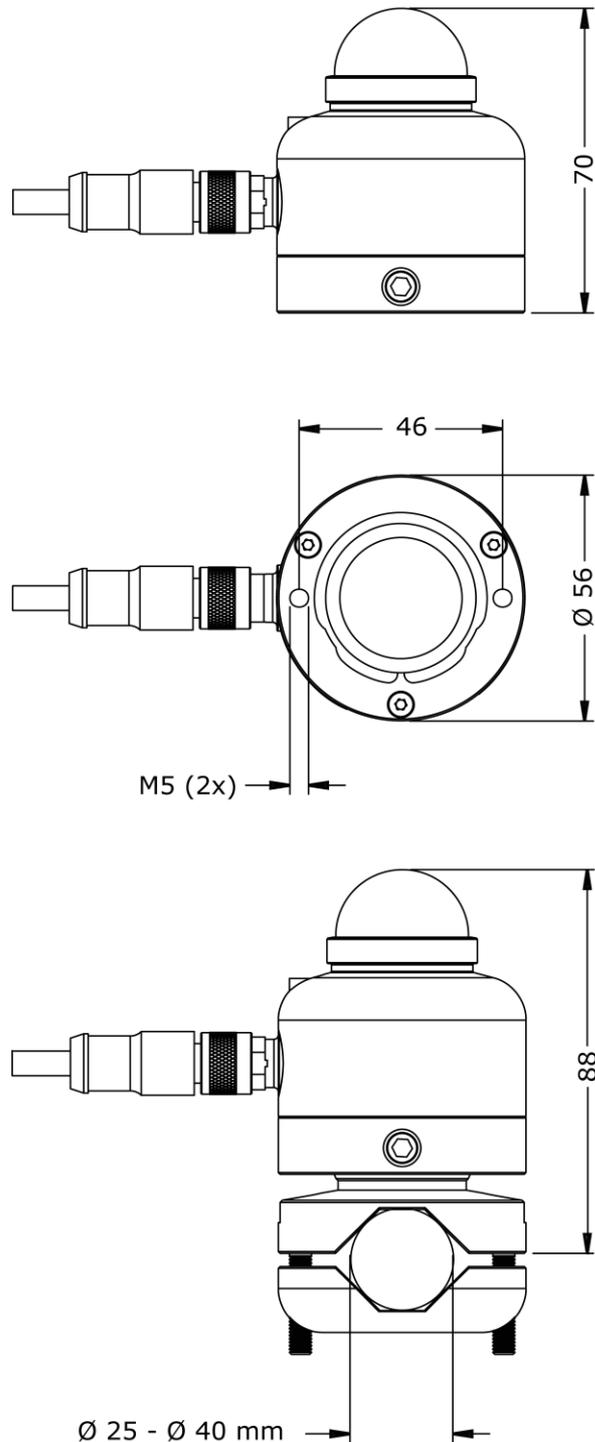
**Figure 3.2.1** Dimensions of SR05 in  $\times 10^{-3}$  m. The bottom drawing shows the height of SR05 combined with its optional ball levelling mount and the tube diameter required for use with SR05's optional tube mount. M5 mounting bolts and the countersunk set screw require a 4 mm hex key for mounting and levelling.
