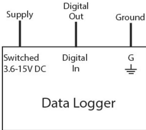
Figure 10: Pigtail End Wiring to Data Logger
