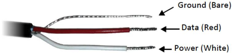
Figure 9: Pigtail End Wiring
