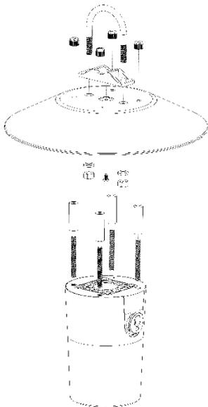
Avoid placing the shield near buildings, paved surfaces, or any other locations which may create a micro-environment significantly different than ambient environment. The World Meteorological Organization (WMO) recommends a mounting height of 1.25 to 2 meters above ground. Air temperature typically decreases with increasing height above the ground surface.
