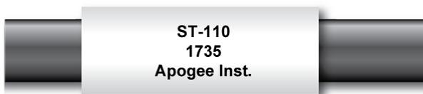
A temperature sensor's model number and serial number are located near the pigtail leads on the sensor cable. If you need the manufacturing date of your sensor, please contact Apogee Instruments with the serial number of your sensor.
