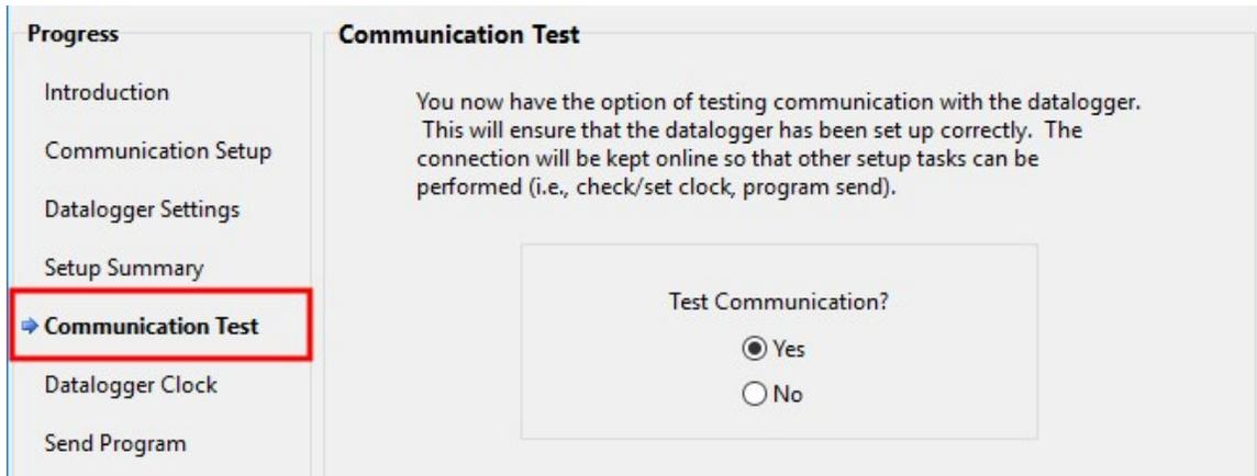
2. Ensure the data logger is physically connected to the computer, select **Yes** to test communications, then click **Next** to initiate the test.
