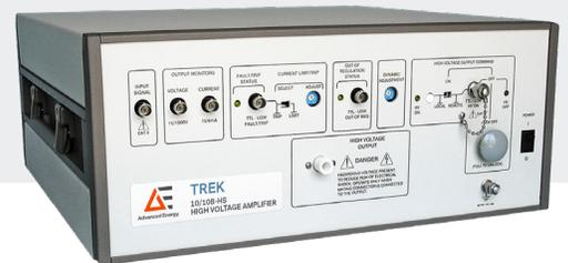
The Trek® 10/10B-HS is a DC stable high-speed, high voltage power amplifier capable of precise control of output voltages. It features an all-solid-state design for high slew rate, wide bandwidth and low-noise operation. The four-quadrant, active output stage sinks or sources current into reactive or resistive loads throughout the output voltage range. This is essential for monitoring the accurate output response and high slew rates when driving reactive loads.
