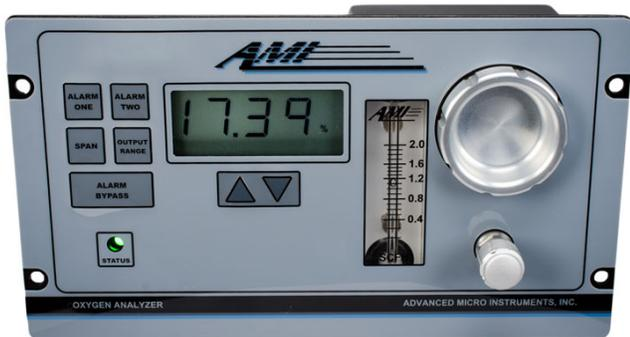
The AMI model 201LC is the ideal solution for measuring percent oxygen in a wide range of applications in a general purpose environment. In a small size, and at very low cost, it provides a complete electronic package and sample system using AMI's patented cell block technology.
