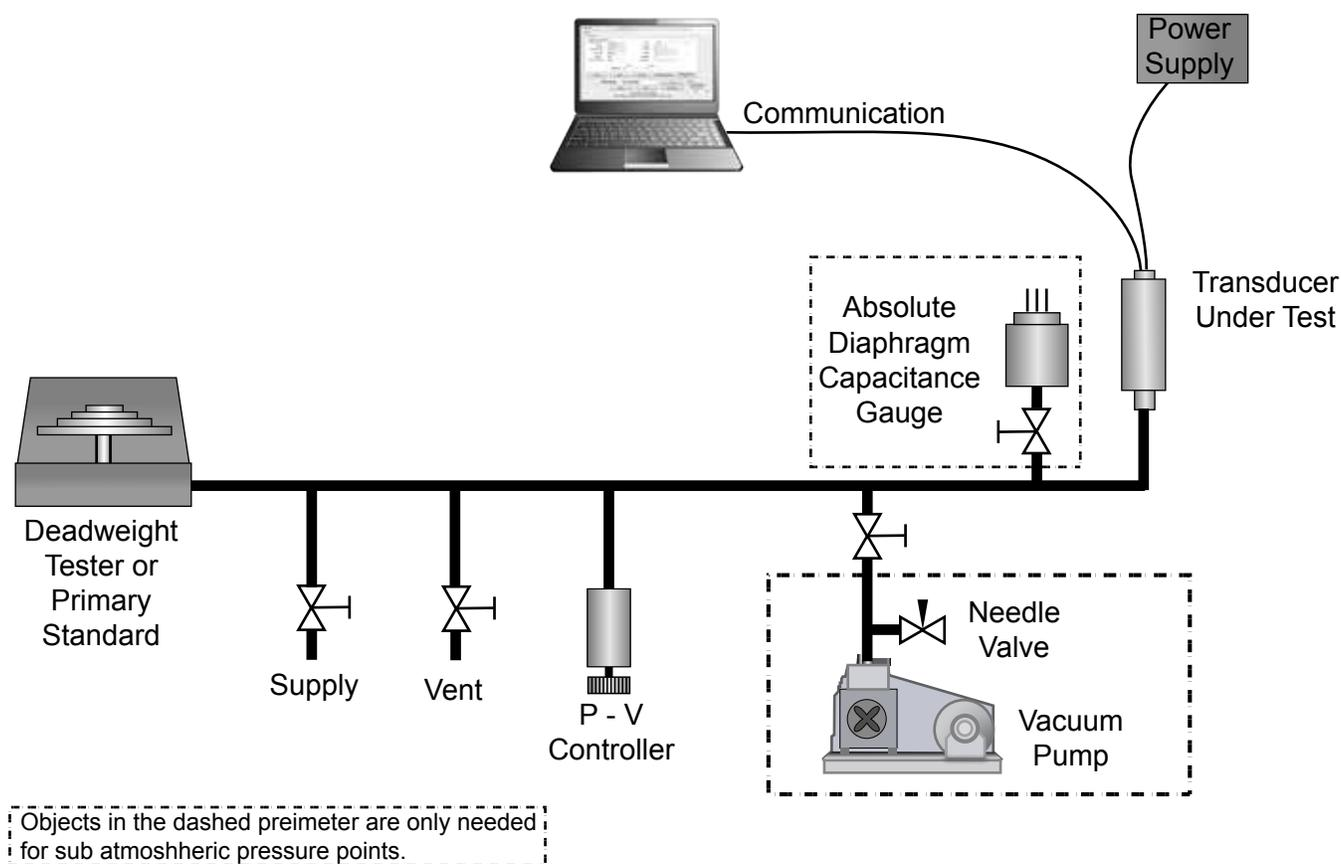
Figure 7.2.5 - Calibration Setup
