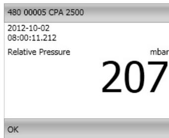
During a running record additionally to the curve a digit display will be shown for each device. Here the measured value and the timestamp of the last measurement will be shown. After recording the display will be closed automatically.
