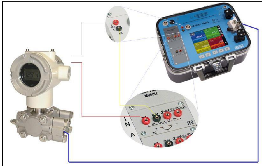
Figure 106 – Pressure transmitter calibration example
