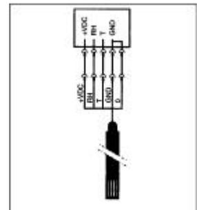
If the five-core cable is prolonged with a five-core cable but concluding with a 4-pin connector, one can connect to this the compensation "0" with the common ground "GND". In this case the cable compensation acts in the five-core cable up to the 4-pin connector.
