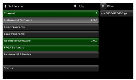
Step2: Tap on the USB icon that appeared. Select "instrument software" from the list. The .gz file copied to the USB drive will appear in a selection on the right-hand side.
