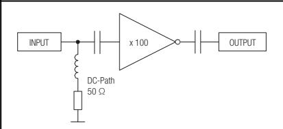
Specifications  $V_s = +15 \text{ V}, T_A = 25^{\circ}\text{C}, \text{ system impedance} = 50 \ \Omega$ Test conditions
