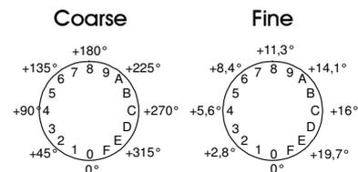
If frequency range  $f > 70$  kHz or 2-f mode is selected, the resolution of digital phase control changes to 2.8  $^{\circ}$  and the phase shift range doubles to 0 ... +720  $^{\circ}$ .
